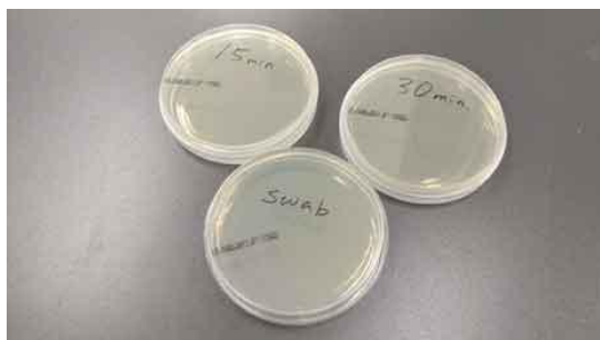
Figure 7. Labeled and sealed agar plates. Air agar plates were labeled '15 min' and '30 min'. Air agar plates were tightly sealed with Parafilm. Swab agar plate was labeled 'swab'.
